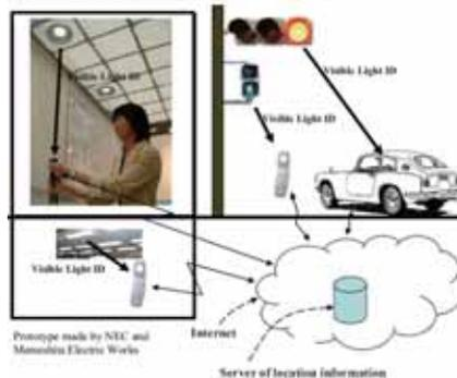
Fig6.1.5. Global location service that uses visible light ID system
