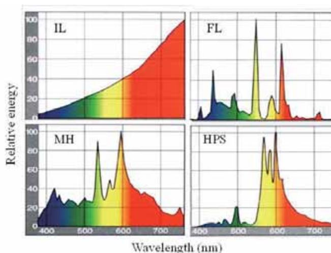
Figure 6.2.1 Spectrum and defects of commonly used artificial light. Incandescent lamp (IL): much heat generation and lack of blue light; Fluorescent lamp (FL): lack of red light; Metal halide lamp (MH): much heat generation and much yellow and green light; High pressure sodium (HPS): lack of blue, green, red and orange light.
