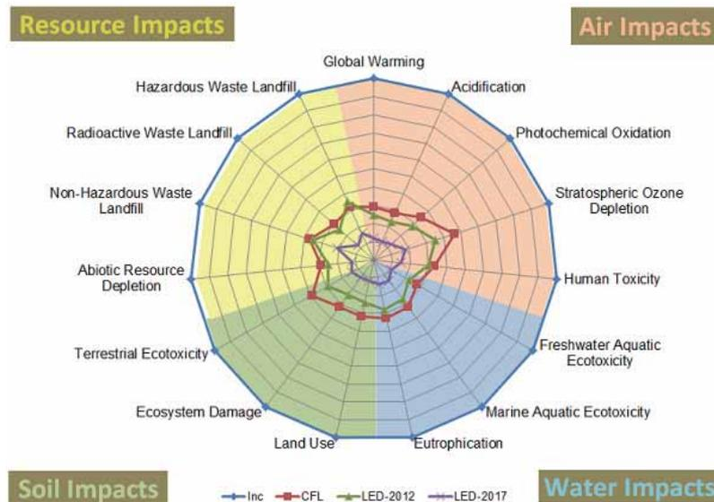
Figure 7.12: Comparison of environmental impact of different light sources normalized to the impact of the incandescent light sources (Scholand, et al., 2012)
