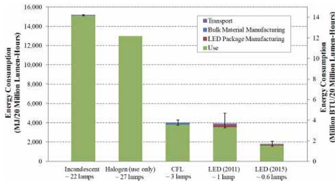
Figure 7.11: Energy consumption and energy needed for transport, material, and product manufacturing. (Solid State Lighting Program. US Dept. of Energy, 2012)
