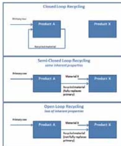
Figure 7.13: Closed loop, semi-closed loop and open loop recycling (Ligthart, et al., 2012).
