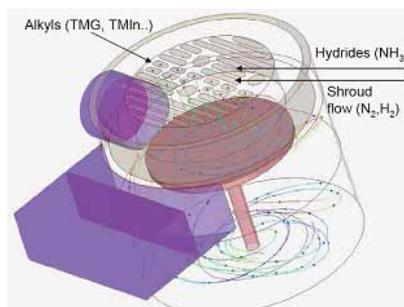
Gas flow model in TurboDisc chamber
