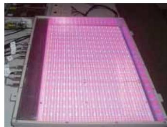
Fig6.2.5 LED light source plate
