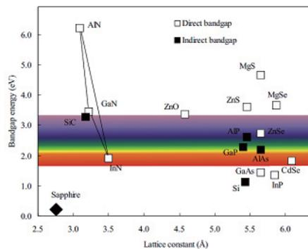
Figure 7.6: Band gap energy versus lattice constant for various semiconductor materials that may create LEDs.
