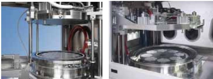
Aixtron's planetary chamber (left) and close coupled showerhead chamber (right).
