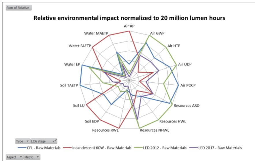
Figure7. 5: Relative environmental impact of different lighting products normalized to 20 million lumen hours and relative to the maximum impact value per category. All data used was obtained from (Scholand, et al., 2012) but reformatted to this figure. The abbreviations are explained in Table7. 2.
