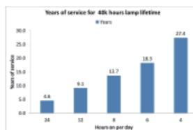
Figure7. 10: Service lifetime in years as a function of hours on per day for a 40k hours lifetime.
