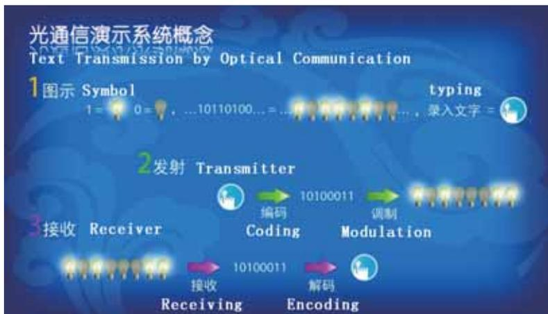
Fig6.1.1 Principle of text transmission by visible lighting communication
