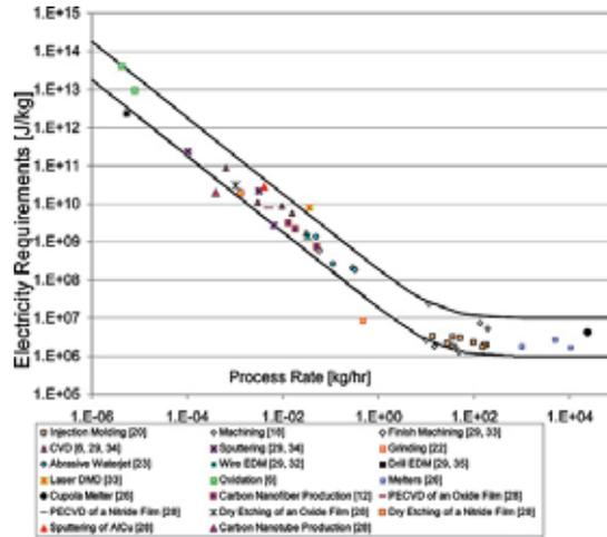
Figure7. 9: Electricity requirements for different production processes. The typical thin film processing technologies have low rate and high electricity requirements (Gutowski, et al., 2009)
