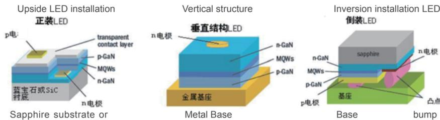
Fig3.3.3: Three LED chip structures
