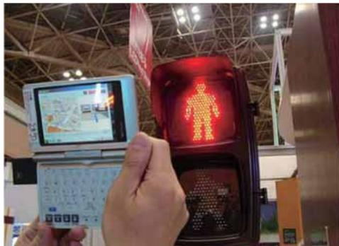
Fig6.1.2 Information broadcast system using LED traffic lights
