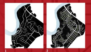
THE ORIGINAL CHONQING MASTER PLAN (FIGURE 1) DISCOURAGED WALKING AND CYCLING. CONSISTENT WITH GLOBAL BEST PRACTICES, THE NEW DESIGN (FIGURE 2) HAS A DENSER GRID OF NARROWER STREETS AND SMALLER BLOCKS THAT PROMOTE CYCLING, WALKING, AND AN ACTIVE STREET LIFE.
