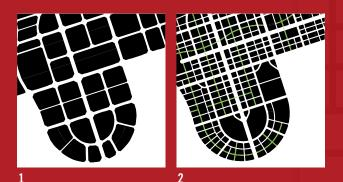
THE ORIGINAL MASTER PLAN FOR CHENGGONG (FIGURE 1) INCLUDED LONG SUPERBLOCKS THAT CATER TO CARS. THE NEW PLAN (FIGURE 2) INCORPORATES A DENSE NETWORK OF STREETS AND PATHS THAT MAKE IT EASIER, SAFER, AND MORE APPEALING TO TRAVEL BY FOOT OR BICYCLE.
