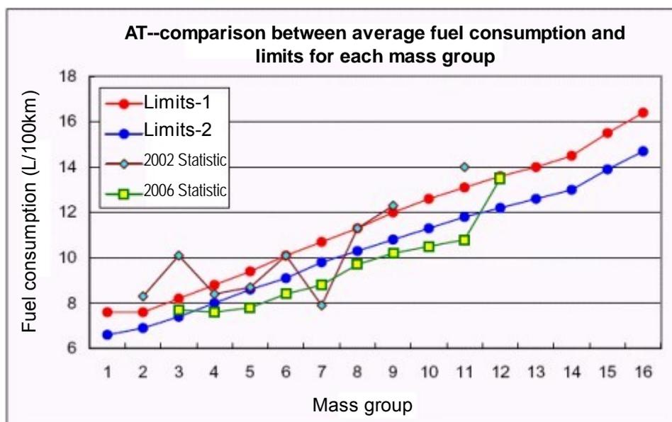
**Figure 2 Comparison between average fuel consumption and fuel consumption limits for each mass group of AT vehicles**
