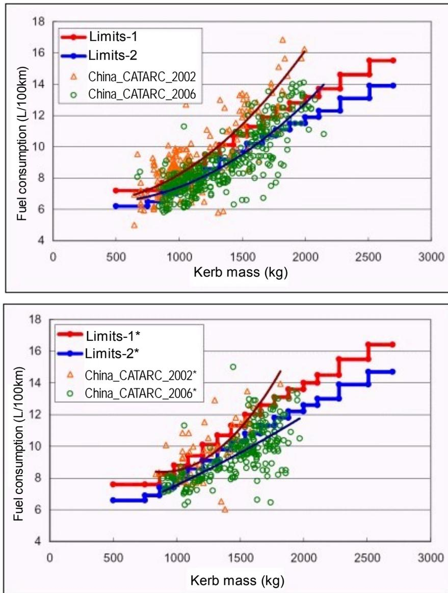
Figure 1 Evolutional trend of mass vs. fuel consumption curve for MT and AT vehicles during 2002~2006
