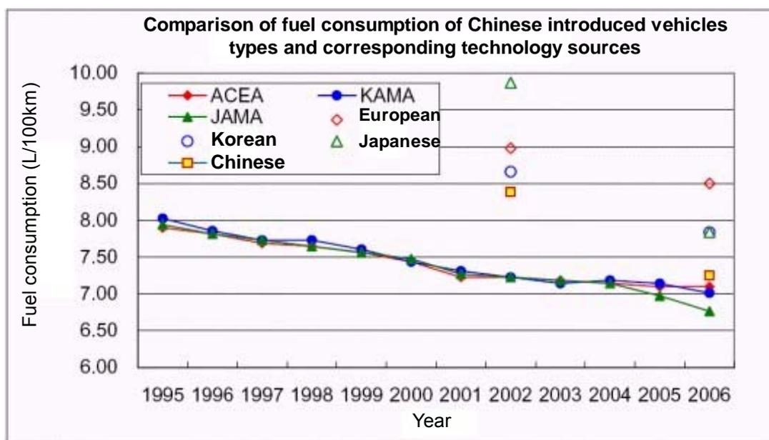
**Figure 7 Comparison of TSAFC corresponding to the vehicle types introduced by China**
