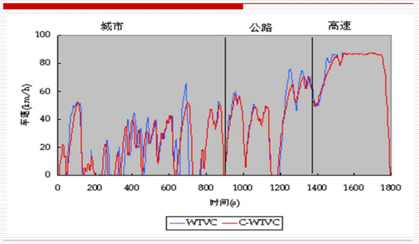
C-WTVC driving cycle, adjusted vehicle and acceleration based on WTVC. Weighted factors were determined based on survey data.
