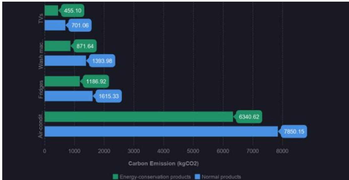
Figure 5 Differences of carbon emission
