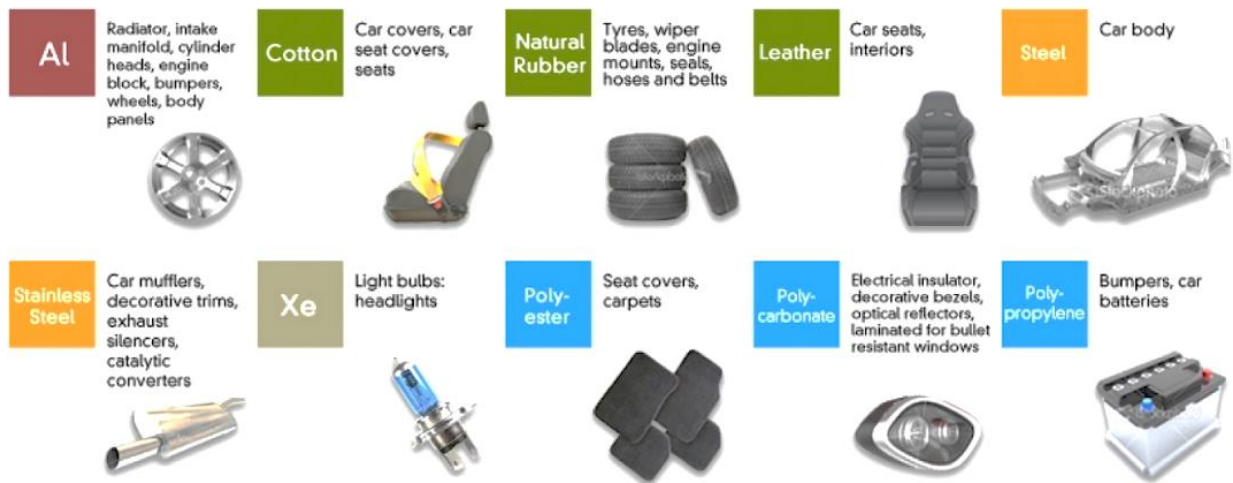
Figure 17 Common materials used in the manufacturing of a car
