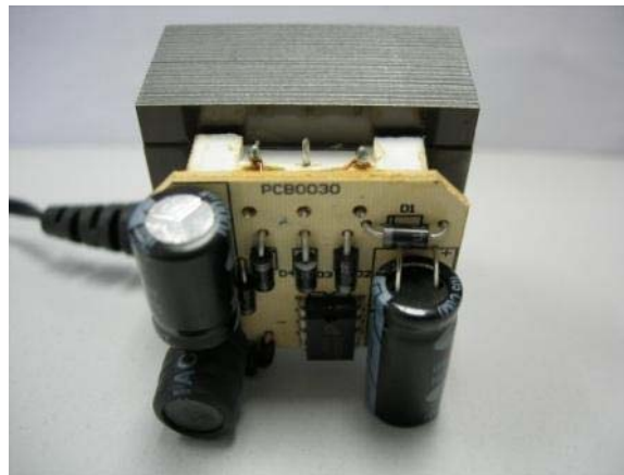
Figure 3: Internal Structure of Linear Mode Power supplies
