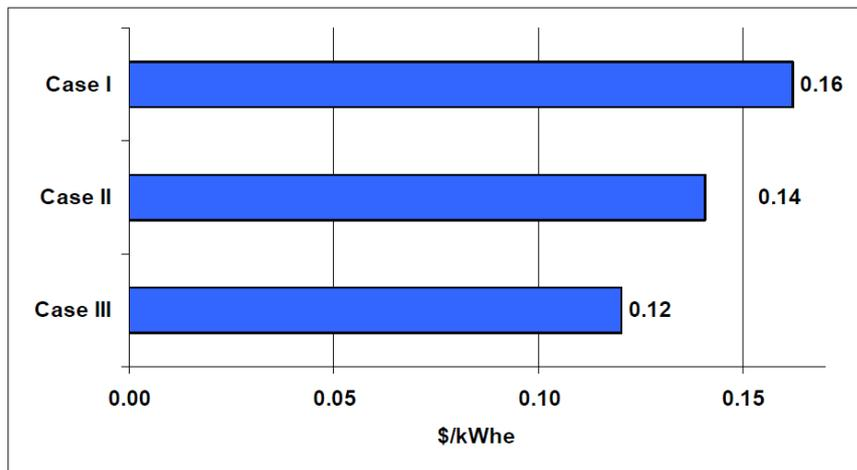
In 2020 the electricity cost of 1000 MW parabolic trough project in China is expected to be reduced at 0.12 \$/kWh, which takes only 75% of the cost for current 100 MW plant.
