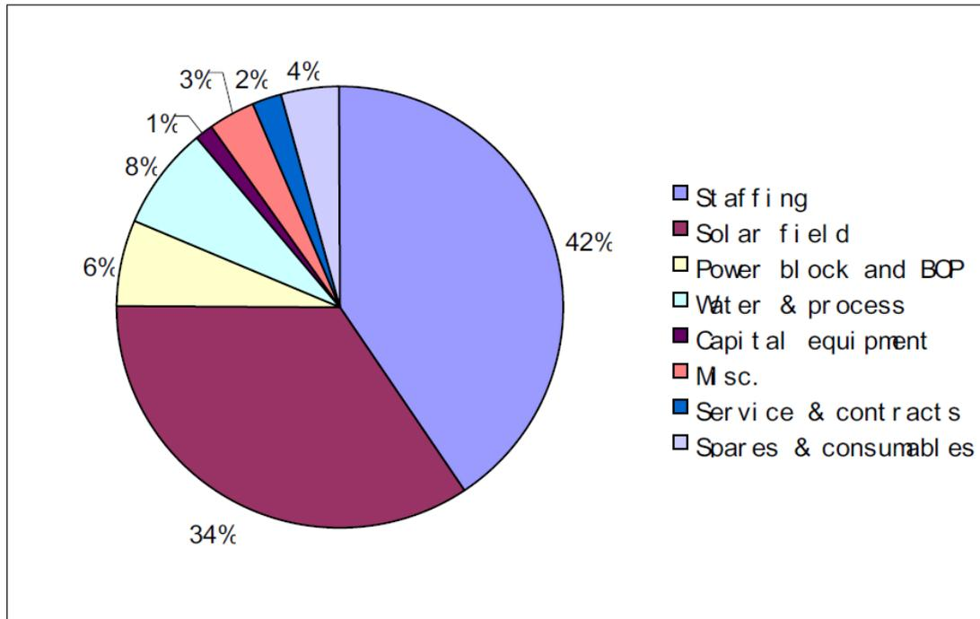
Based on Figure 6, it is evident that the largest component of the O&M costs is the staffing costs. The following table 10 shows a comparison of the staffing costs for China and Germany.
