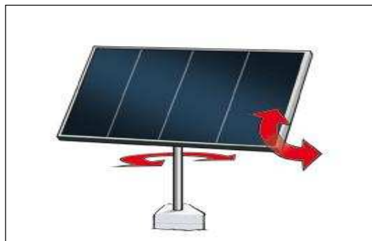
Figure 2-12: Dual axis optical solar tracking /Heliotrack 2009/
