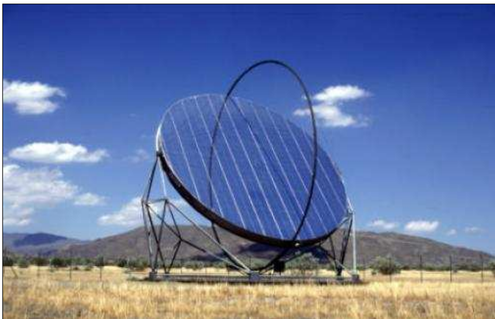
Figure 2-14: Membrane heliostats /Thomas 2000/
