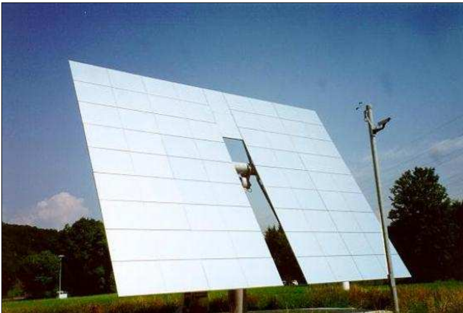
Figure 2-13: Faceted glass/metal heliostats /Thomas 2000/
