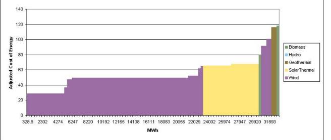
Supply curve ranks the adjusted cost of a portfolio of resources to a load zone in the WREZ model
