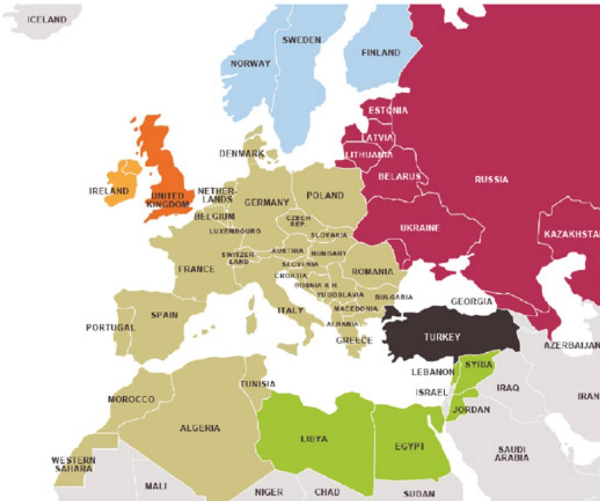
(\*) Electrical synchronism is the term used where power grids in different countries share the same electrical frequency (measured in Hertz or Hz).
