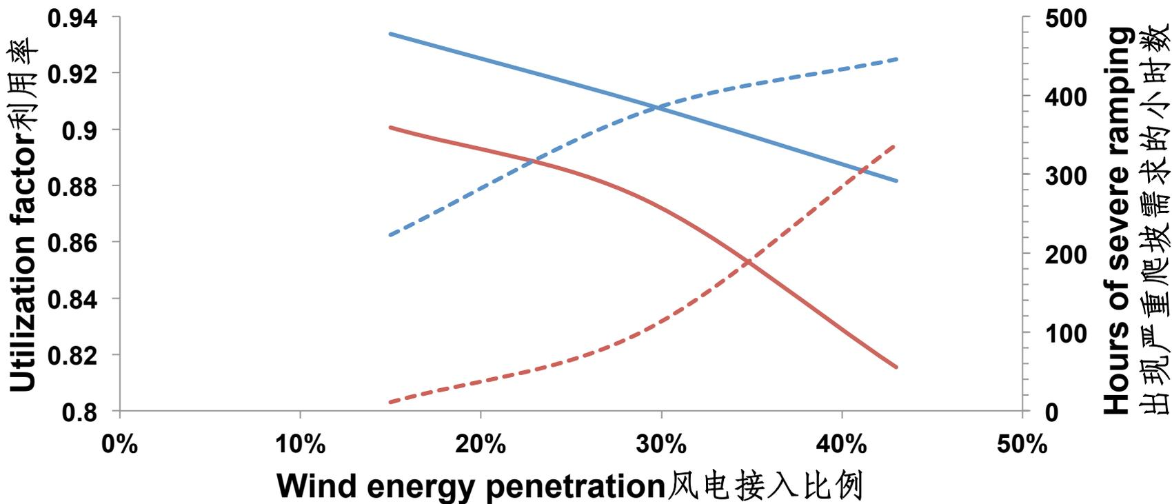
— CCGT utilization factor    — Coal utilization factor    - - - CCGT ramping    - - - Coal ramping
